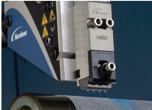
Universal Summit nozzles control adhesive fiber size, density and pattern width for better bond performance.
